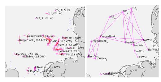
Possible hub-connected OWPP investments, and some example connections in the meshed scenario
